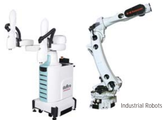
duAro collaborative dual-arm SCARA robot (Photo: provided by Kawasaki Heavy Industries, Ltd.)
