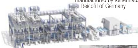
Spunbond production line manufactured by Reifenhäuser Reicofil of Germany
