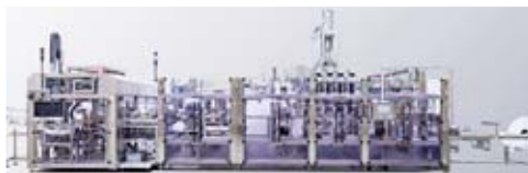
Form-fill-seal (FFS) machine manufactured by SACMI of Italy
