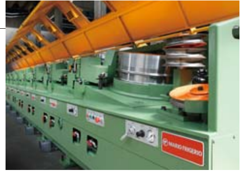
Wire drawing machine of Mario Frigerio, Italy
